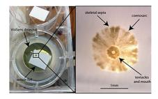
The calcified skeleton of corals makes it difficult to take biological measurements. The VisiSens imaging system was applied to measure oxygen consumption patterns in individual corals immediately after settlement and initiation of calcification. Furthermore, the difference in oxygen consumption between corals exposed to ambient or low pH conditions, which mimic future ocean acidification, was investigated.
